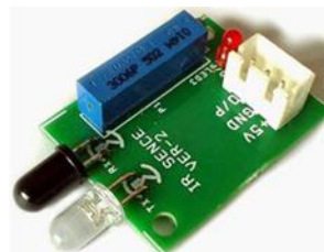
FIGURE 3.1 IR Sensor principal of IR sensor
