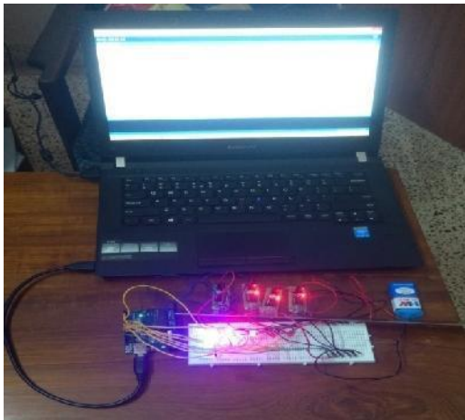
FIGURE 4: The Automatic Street Light Control Based on Vehicle Detection Using Arduino.
